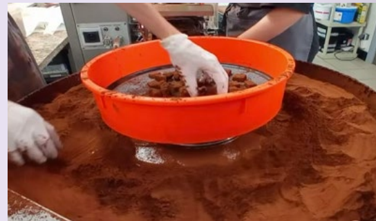
FIGURE 2 Simulation (Béguin, 2013; Daniellou, 2007; Van Belleghem, 2018) of a sifting device and reduced turntable speed, eliminating the rebalancing gesture, co-designed by/with operators.
