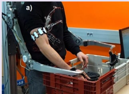
FIGURE 2 Upper-limb BHV2 exoskeleton used for myoelectric control (Treussart et al. , 2019).
