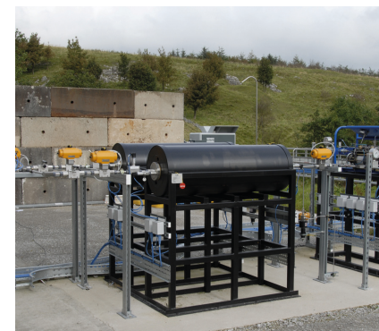
Net zero emission: Test with high pressure hydrogen at HSE. Copyright HSE.
