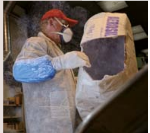
▲ Figure 10. Filling a reaction vessel during formulation of a glue
