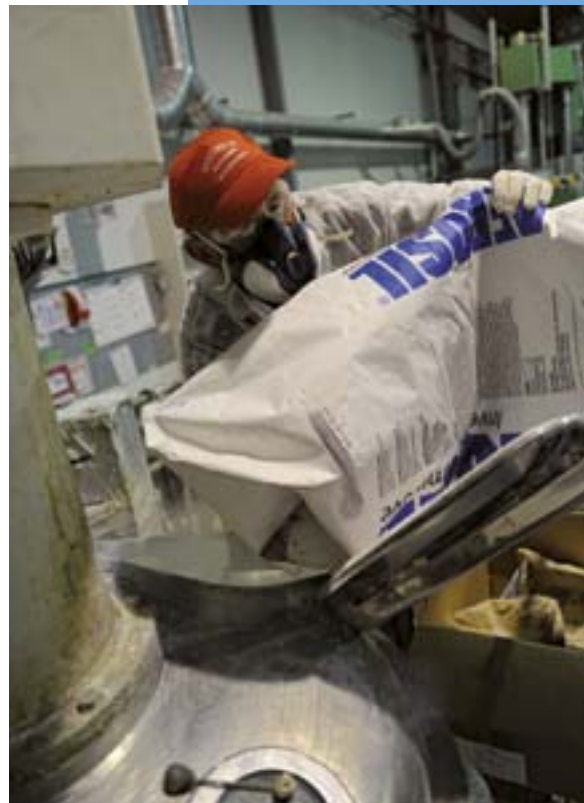
▲ Figure 30. Empty containers should be treated as nanomaterial waste
