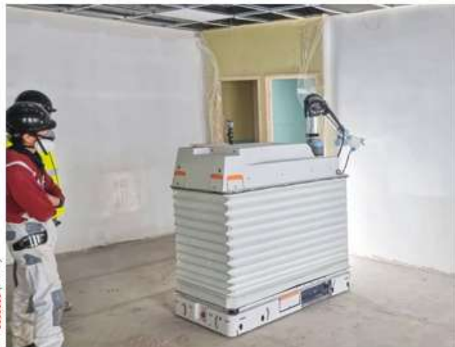
Paco, the paint and sanding robot on wheels.
